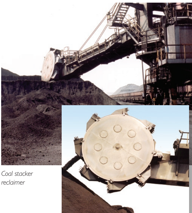
Typical stacker reclaimer bucket wheel during inspection for potential bearing conversion
