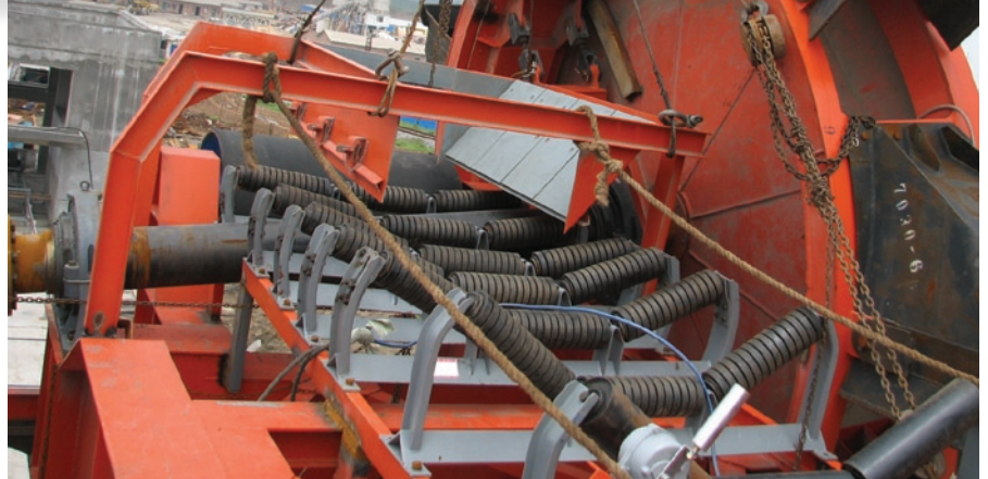
Cooper bearing on a stacker reclaimer in China
