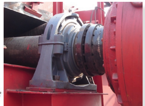
Cooper bearing on a newly built stacker reclaimer in China
